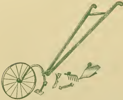
Fig. 4—Wheel hoe and hand cultivator, to be had with attachments such as plow, cultivator teeth, shovels and rake. A simple form may be made at home.
